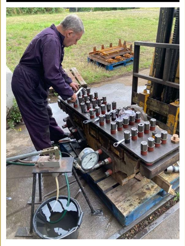
The paid engineering staff and contractors work closely with volunteers to deliver testing and refurbishment of components for *Tornado*. From work on the smoke box door to the hydraulic testing of the superheater header (pictured above), the team are working hard on Tornado's overhaul. Read more here.
